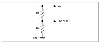
Figure 2. Setting the Input Undervoltage Lockout
