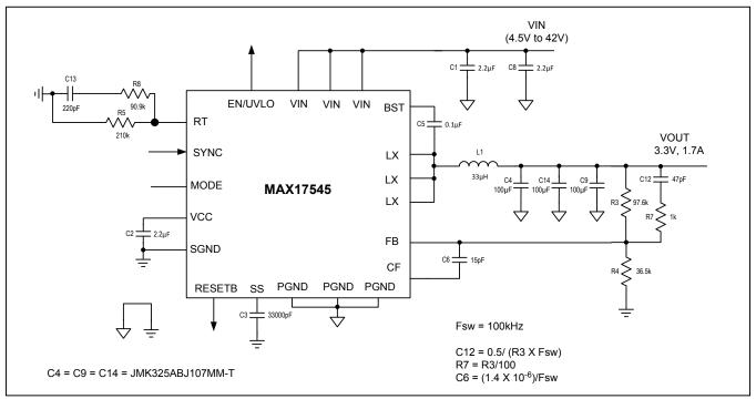
Figure 5. 3.3V Output, 100kHz Switching Frequency
