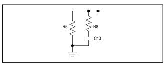
Figure 1. Setting the Switching Frequency
