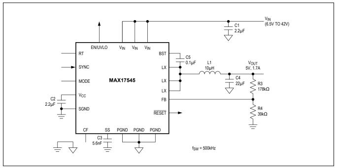
Figure 4a. 5V Output, 500kHz Switching Frequency
