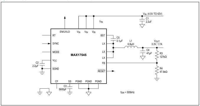
Figure 4b. 3.3V Output, 500kHz Switching Frequency
