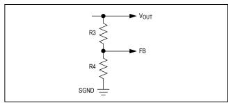
Figure 3. Setting the Output Voltage
